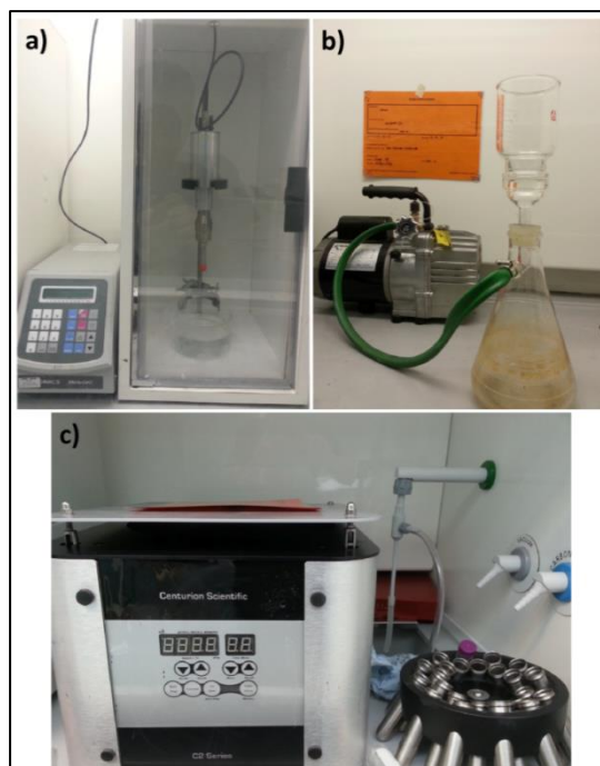
Figure 3.2 shows: a) the ultrasonic probe; b) vacuum filtration setup and; c) centrifugation machine.
