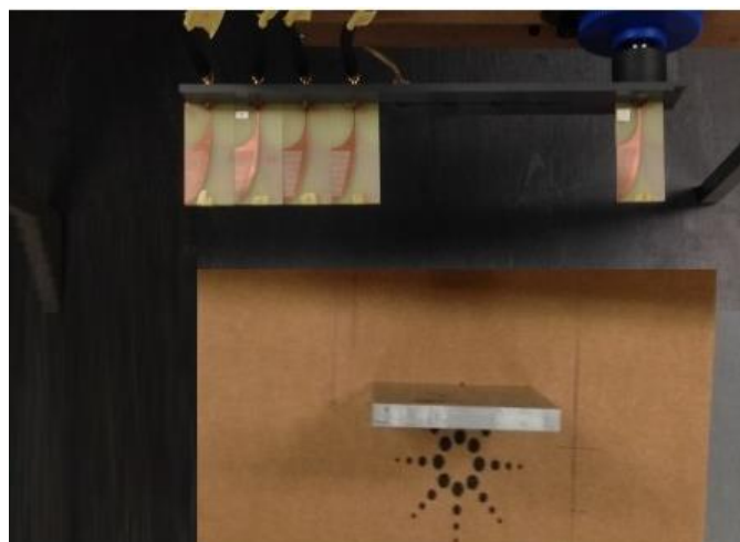
Figure 5-3 One metallic target placed at a certain distance away from the array in experiment
