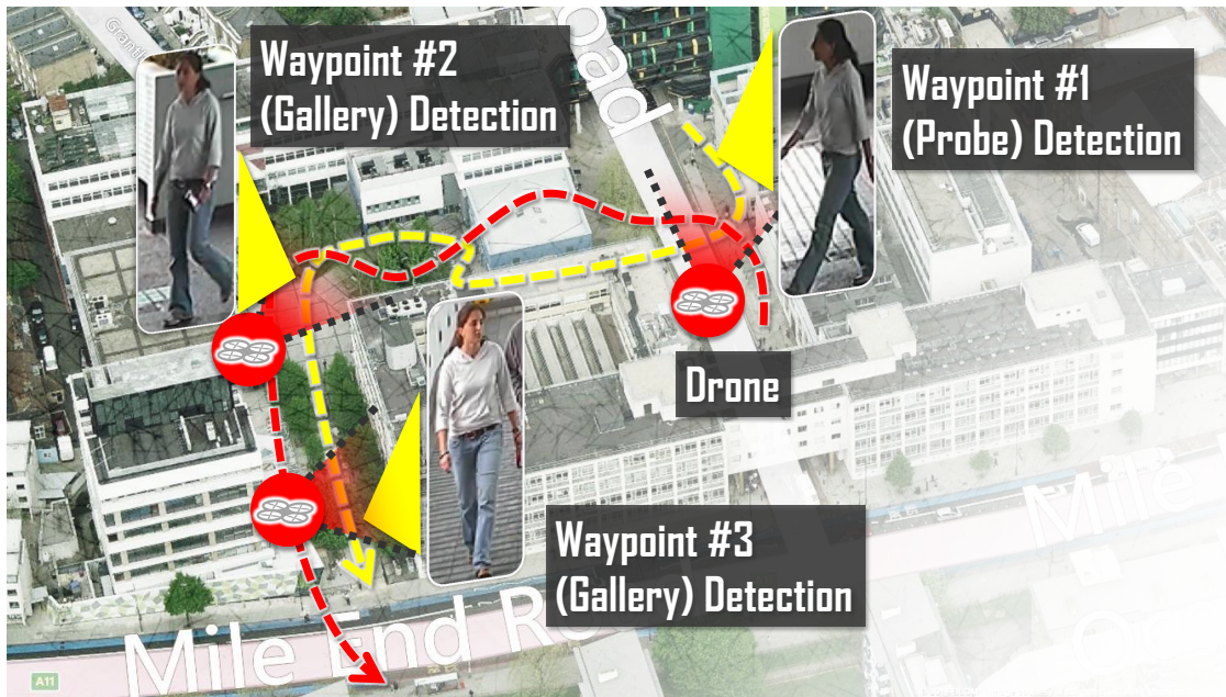
Figure 6.4: Illustrative example of a real-world re-identification set-up using a mobile re-identification platform (MRP), or UAV. Contrasting with the same scenario using static CCTV (Figure 6.3 on the preceding page), the UAV is able to follow (red path) the path of the person (yellow path). This enables surveillance in areas with no existing CCTV coverage, but at the cost of person detections that are more diversified in terms of their appearance and their appearance under the effect of practical covariates such as viewing angle and lighting conditions.
