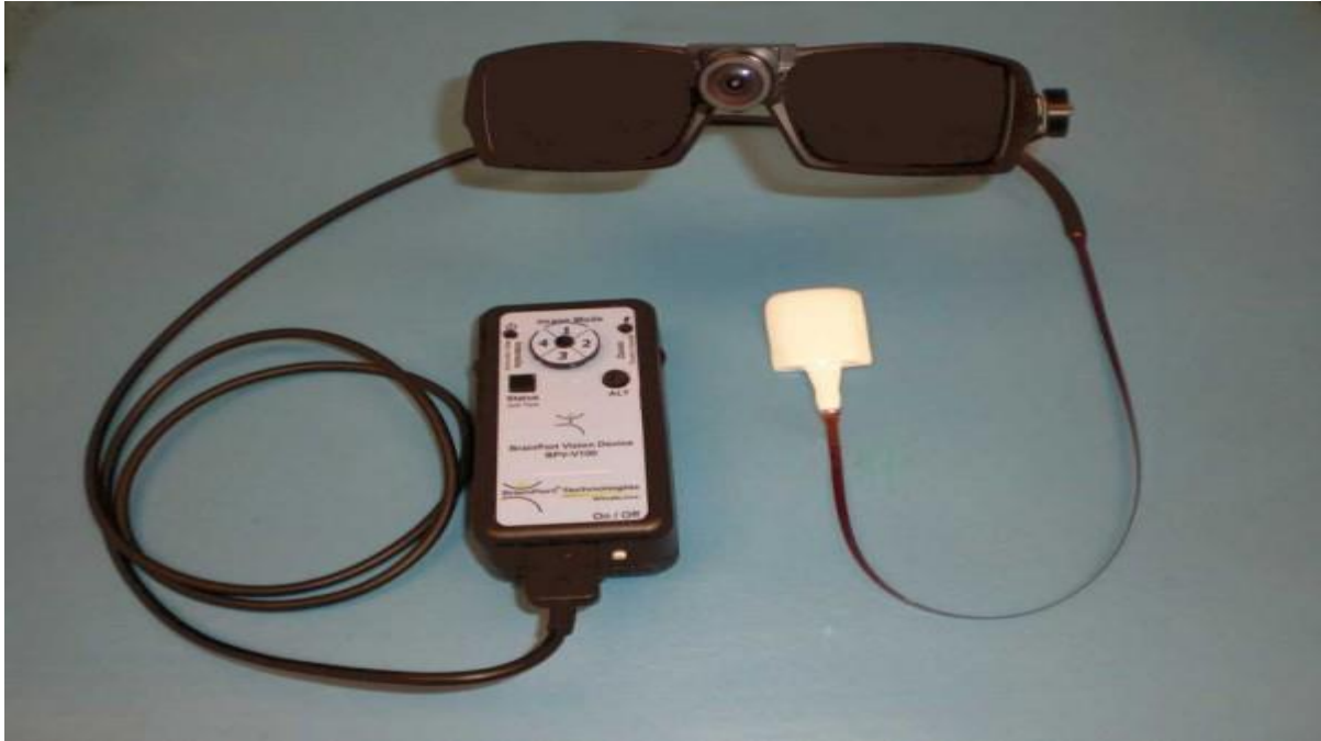
Figure 1.3: The hardware components of the Brainport TDU. The sensor is mounted central on the glasses with the transmitter as 20x20 array of vibro-tactile solenoids. Image taken from (Y. Danilov & Tyler, 2005)
