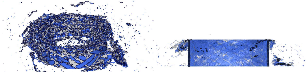
Figure 5.22: Deformation of the wound tube in crash loading obtained by simulation t=12 ms.
