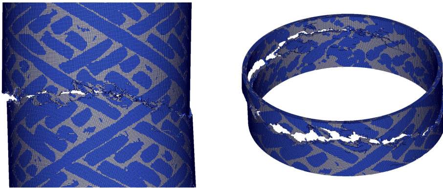
Figure 5.7: Fracture of wound tube under tensile loading.
