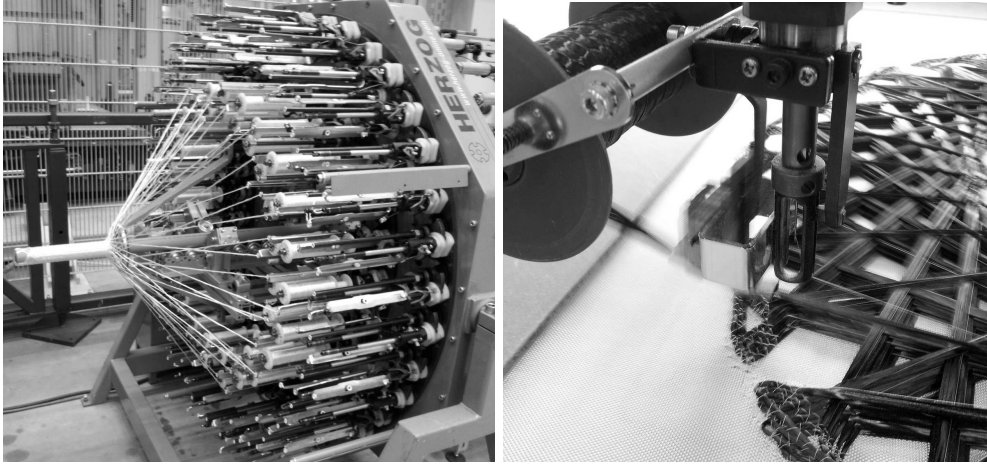
Figure 1.3: Manufacturing of composite structures by a) braiding and b) tailored fibre placement.
