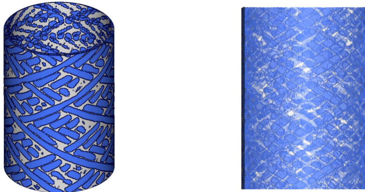
Figure 5.10: Deformation of the wound tube in crash loading obtained by simulation t=0 ms.
