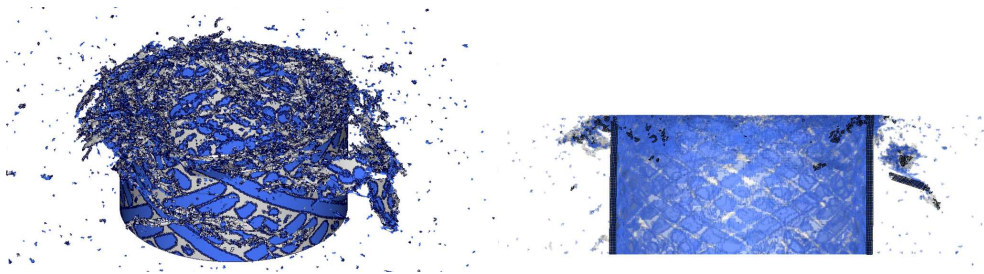
Figure 5.19: Deformation of the wound tube in crash loading obtained by simulation t=9 ms.
