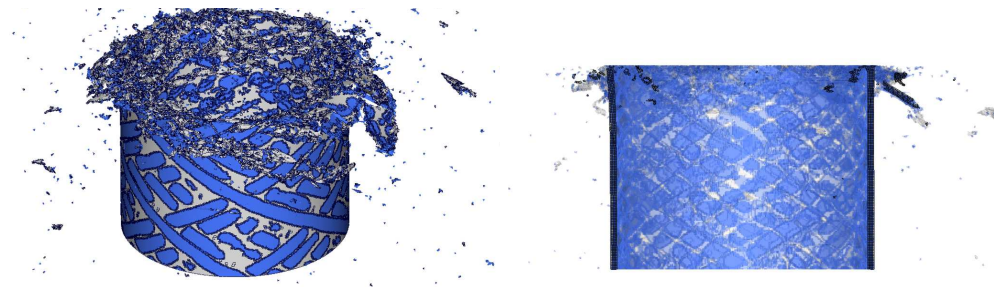
Figure 5.16: Deformation of the wound tube in crash loading obtained by simulation t=6 ms.
