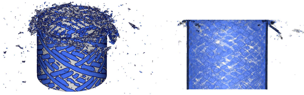
Figure 5.15: Deformation of the wound tube in crash loading obtained by simulation t=5 ms.
