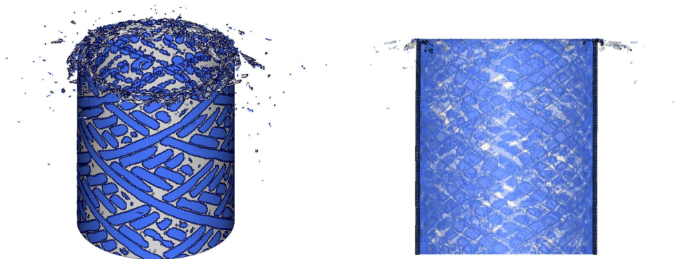
Figure 5.12: Deformation of the wound tube in crash loading obtained by simulation t=2 ms.
