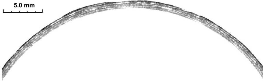
Figure 3.10: CT record of complete component (filament wound tube specimen for dynamic testing) - section cut upper part.
