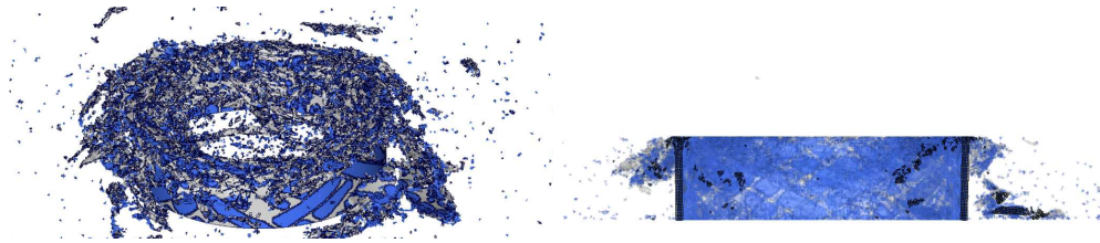
Figure 5.23: Deformation of the wound tube in crash loading obtained by simulation t=13 ms.
