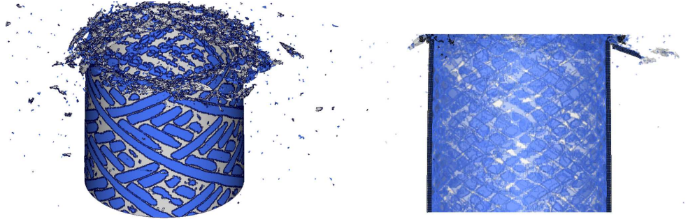
Figure 5.14: Deformation of the wound tube in crash loading obtained by simulation t=4 ms.
