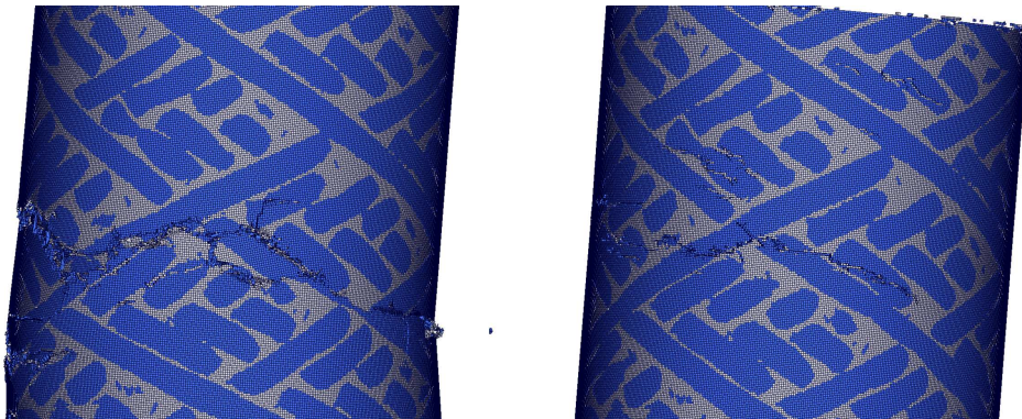
Figure 5.8: Fracture of wound tube under compressive loading.
