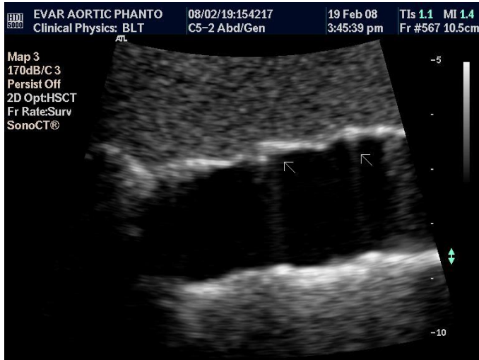
Figure 35: Longitudinal ultrasound B-mode image produced of the EVAR stent (large flow system) within the EVAR phantom
