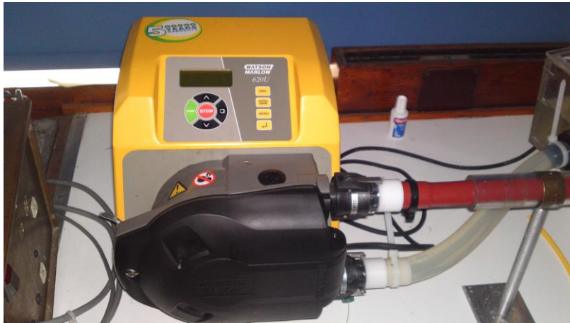
Figure 11: Doppler blood-mimic fluid leaves the reservoir and enters the dual band pump, achieving pulsatile flow
