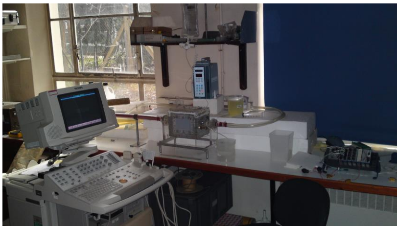
Figure 7: The laboratory set up of ultrasound machine and phantom with two independent flow systems
