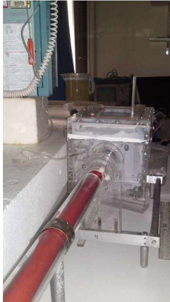
Figure 13: Proximal entry flow to the EVAR phantom
