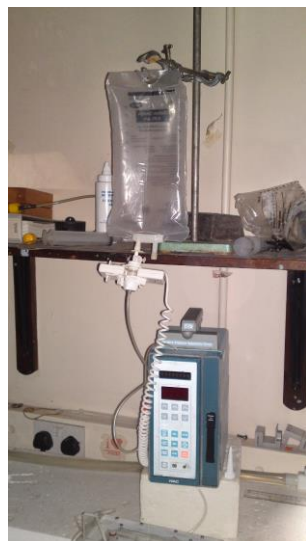
Figure 18: Empty saline bag reservoir for the small flow system that enters a fluid pump to produce the variable endoleak
