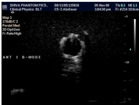
Figure 40: Images of the phantom simulated endoleak in an anterior position 1, using B mode, colour Doppler and contrast enhanced ultrasound
