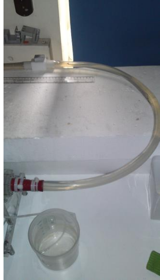
Figure 28: Large flow system curves in a circle after leaving the phantom. Along its course an injectable inlet allowed administration of contrast ultrasound to the system
