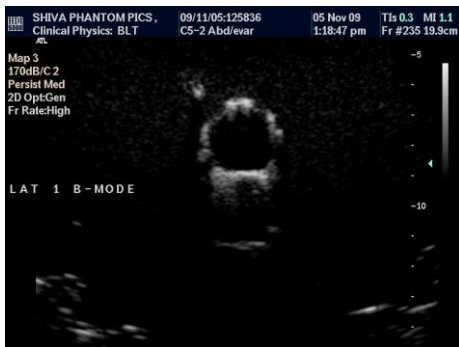
Figure 45: Images of the phantom simulated endoleak in a lateral position 1, using B mode, colour Doppler and contrast enhanced ultrasound
