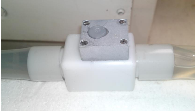
Figure 30: Injectable inlet for large system contrast administration
