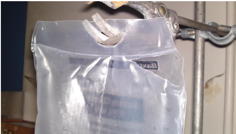
Figure 31: Small flow system reservoir bag cut at one end to refill Doppler fluid from the Perspex beaker and administer contrast
