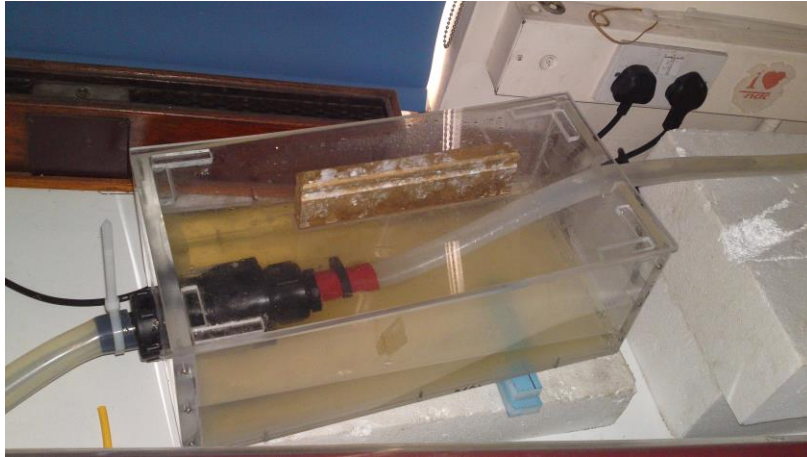
Figure 9: Doppler blood-mimic reservoir of the large (EVAR stent) flow system
