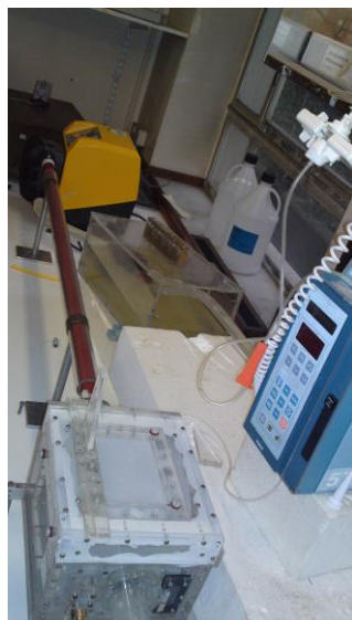
Figure 12: Fluid flows from the pump to the EVAR phantom, rate of 90bpm
