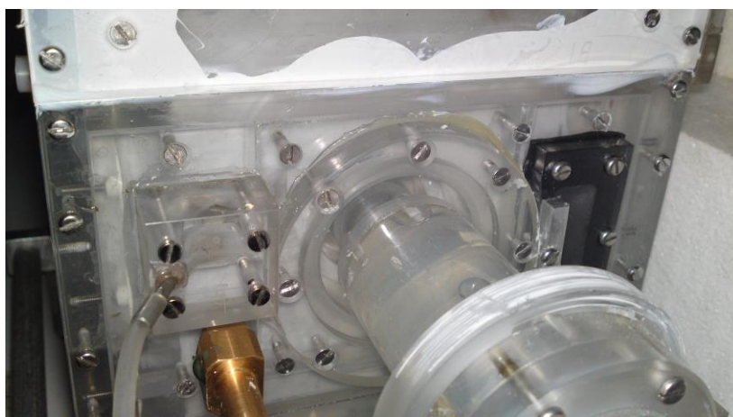
Figure 24: Distal aspect of the phantom showing the large and small flow systems exiting the housing
