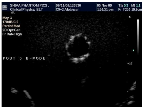
Figure 52: Images of the phantom simulated endoleak in a posterior position 3, using B mode, colour Doppler and contrast enhanced ultrasound
