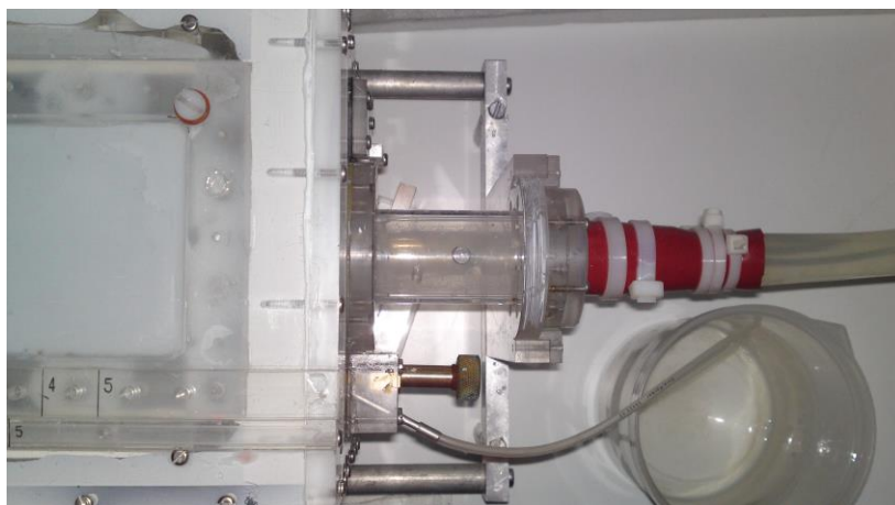
Figure 23: Distal aspect showing the large and small flow systems exiting the housing. The small system collects into the Perspex beaker and is manually used to replenish the small system reservoir in the saline bag
