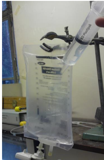
Figure 32: Filling the small flow system reservoir bag with Doppler fluid
