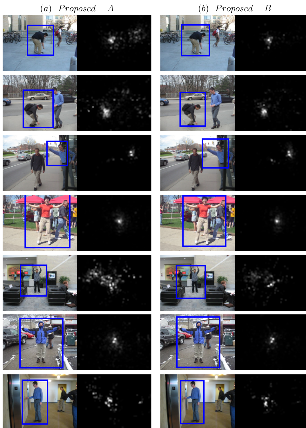
Figure 5.7.: Some detection results on CMU dataset: (a) First column shows the detected bounding boxes and the corresponding spatial Hough space for the method Proposed – A . (b) Second column shows the detected bounding boxes and the corresponding spatial Hough space for the method Proposed – B . We can see that modelling the background significantly reduces the background clutter and increase the votes at the center location of the object
