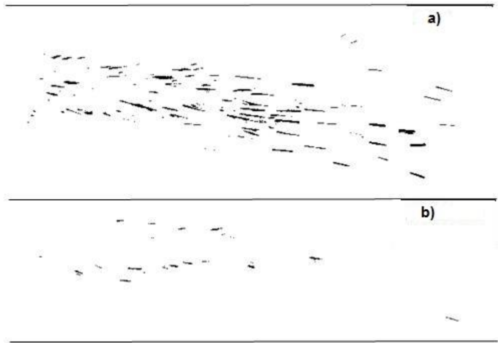
Figure 3.73 Binarised images of the particles of Si (720 nm (a) and 1 \mu m (b) ) showing the higher ignitibility (reactivity) of the particles having a smaller diameter.
