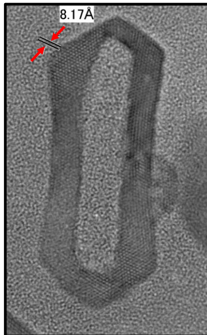
Figure 3.6: TEM image of enamel crystal showing dissolution at the centre of the crystal (Yanagisawa and Miake, 2003)
