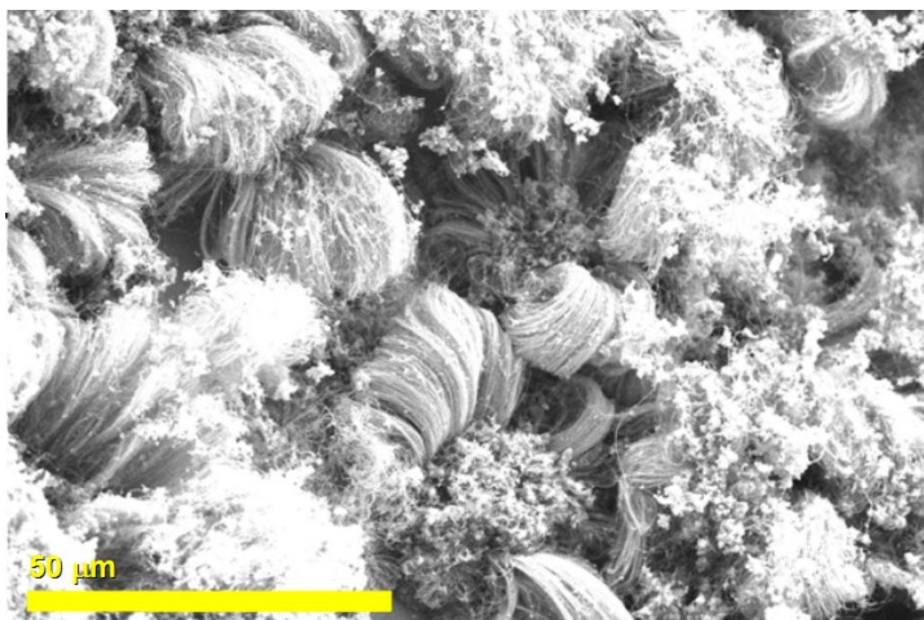
Fig.77: Scanning electron micrograph (taken at 20 kV) showing the homogeneity of the flower-like structures grown in the new substrate.
