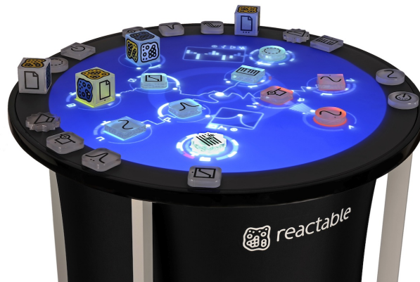
Figure 2.7: The Reactable with a number of its marked objects above the translucent surface onto which the visual feedback is projected. (Photo: Massimo Boldrin. Reproduced with permission.)
