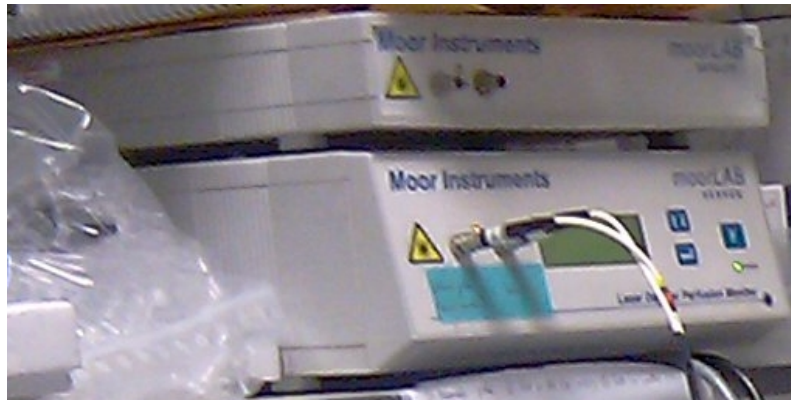
Figure 2.12 MoorLAB Doppler processing units.
