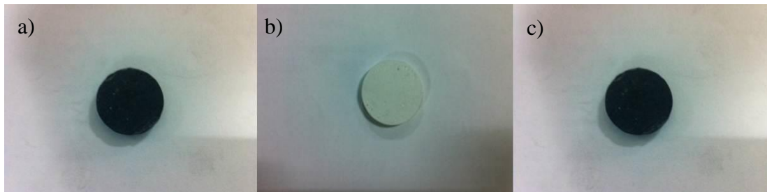
Figure 4.2: Photos of ceramic disc: (a) after sintering; (b) after air annealing; (c) after reduction
