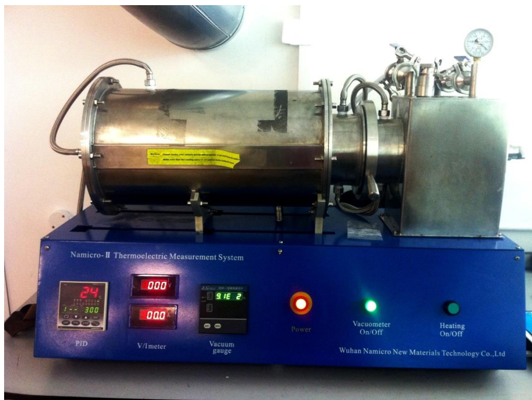
Figure 3.5: Lab built (in China) electrical resistivity and Seebeck coefficient measurement system
