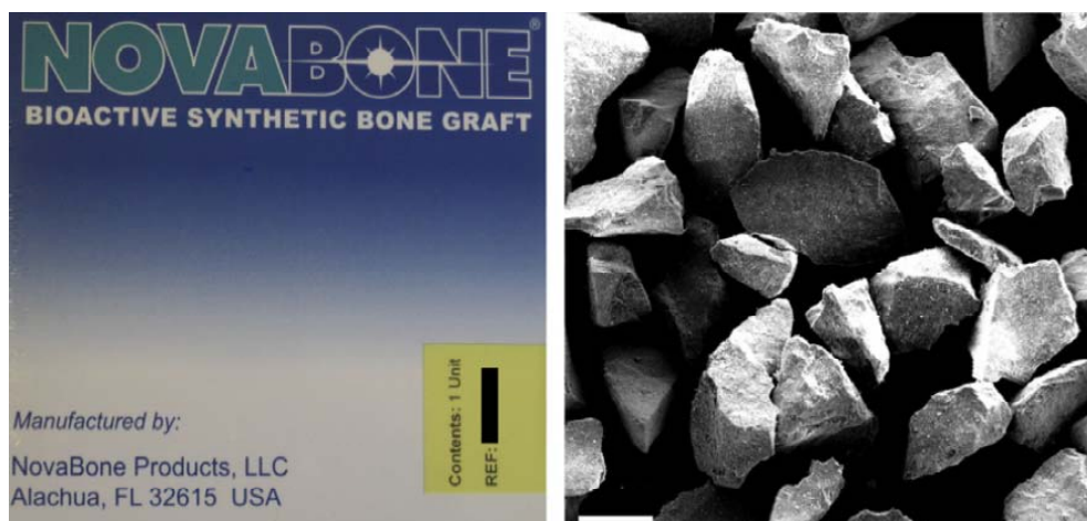
Fig.1. 3. NovaBone packaging, with an SEM image of the particles. Scale bar is 200\ \mu\text{m} 20 .
