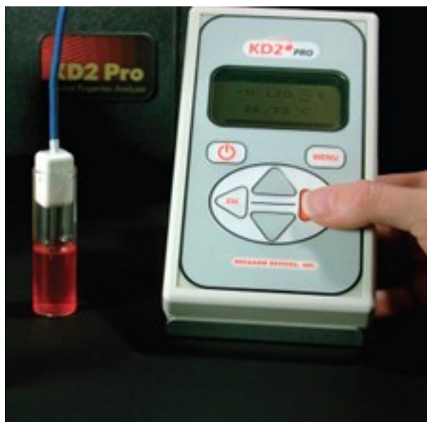
Figure 4-1 scheme of thermal conductivity measurement by KD2 probe
