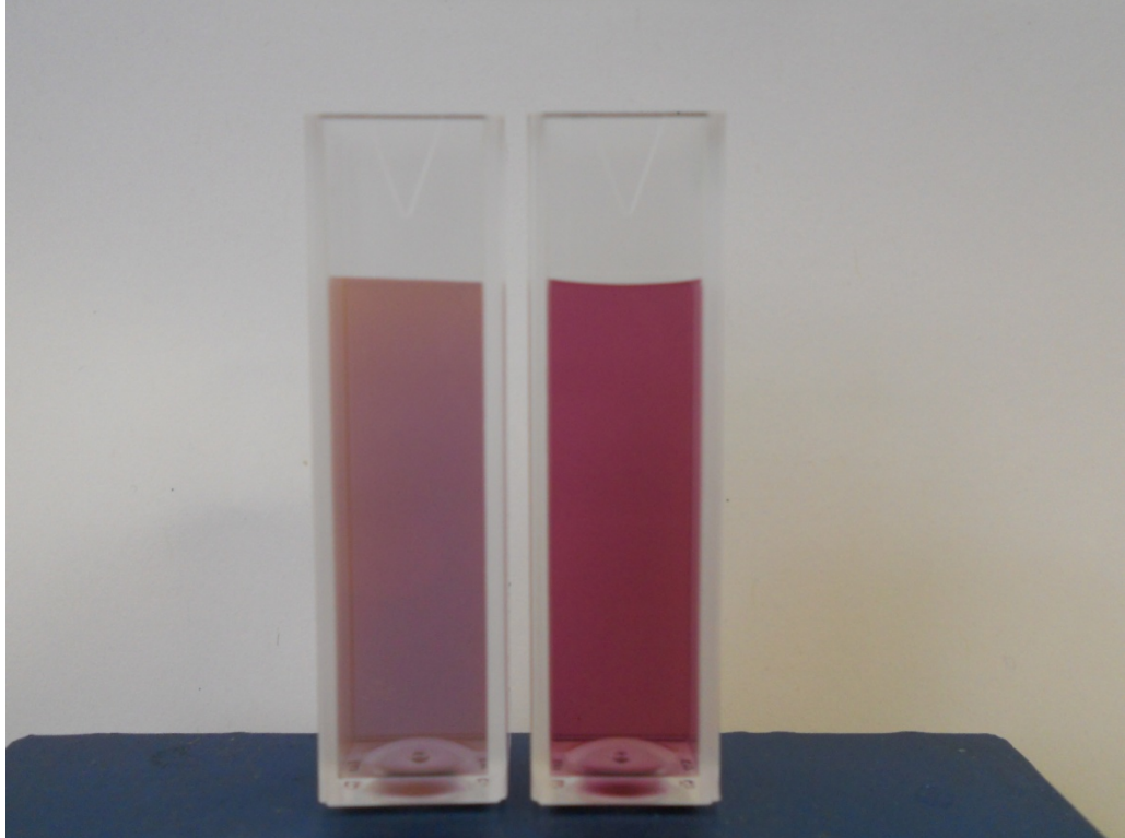
Figure 3-8 The colour of 90 nm gold nanoplates (left) and 90 nm GNPs (right)
