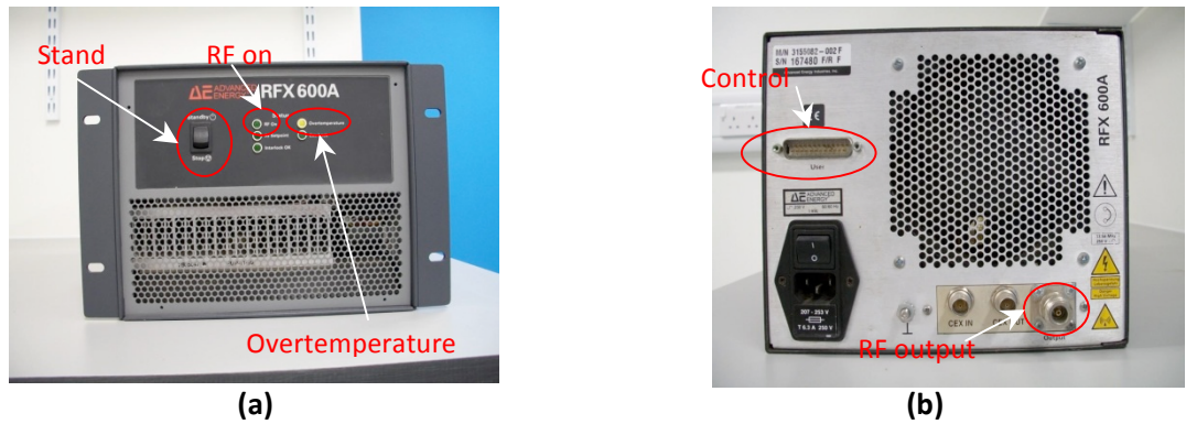
Figure 4-14 13.56 MHz high power generator. Advanced Energy Industries, Inc. Module RFX 600A. (a) Front panel; (b) Rear panel.
