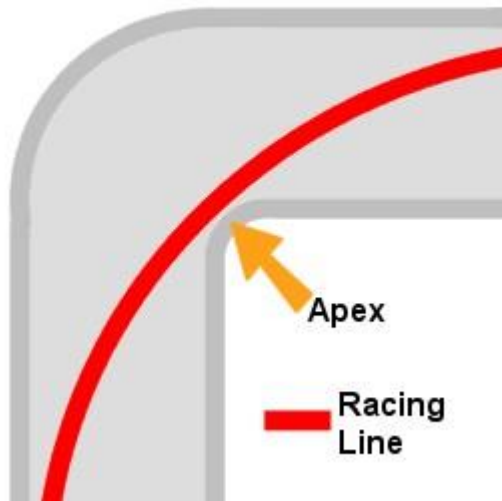
Figure 2.3: Diagram of the racing line through a corner, along with its Apex. (Driving Experiences, 2012)
