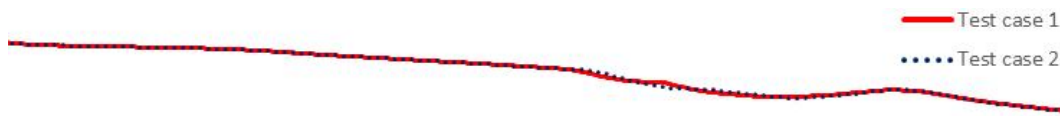
Figure 5.6: Comparison of lines from stationary collision avoidance testing. From this comparison, it can be seen that both AI moved out by the same amount in order to get passed the stationary vehicle, despite test case 2 (dark blue, dotted) having more width to avoid than test case 1 (red, solid.)
