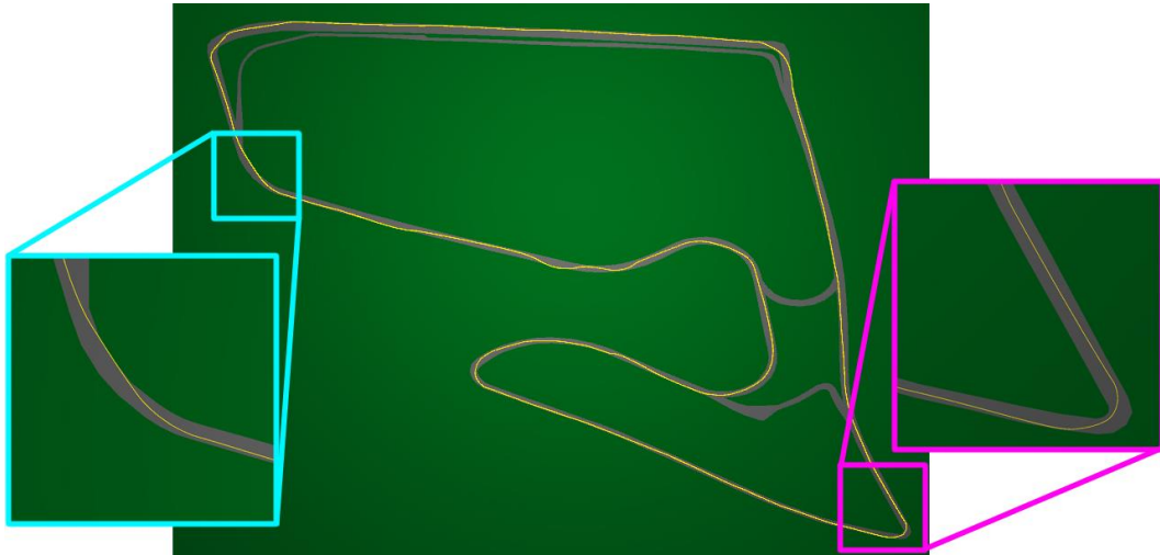
Figure 3.2: Line Drawn by the AI of the Sector based system. Notice how the line taken by the AI in the corner highlighted in blue isn't a consistent curve, with the AI going straight for the corner itself.
