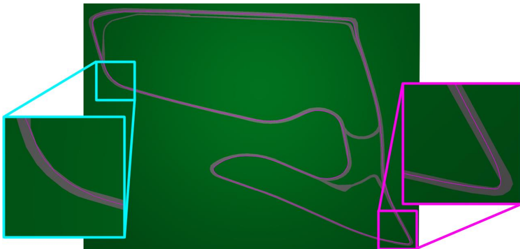
Figure 3.5: Line Drawn by the AI of the Sensor based system. Notice how the line taken by the AI in the corner highlighted in blue is a consistent curve than that of the sector method, while the corner highlighted in the pink box shows the car entering and exiting the corner within the centre of the track rather than the edge.
