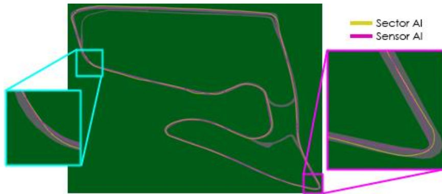
Figure 3.7: Lines drawn by the sector and sensor methods. The two highlighted corners methods show the strengths and weaknesses of each of the two methods. The sector method is able to use appropriate lines through the straights as well as corner entry and exits (yellow) while the sensor method is able to take the cornering lines better, finding the apexes every time (pink.)
