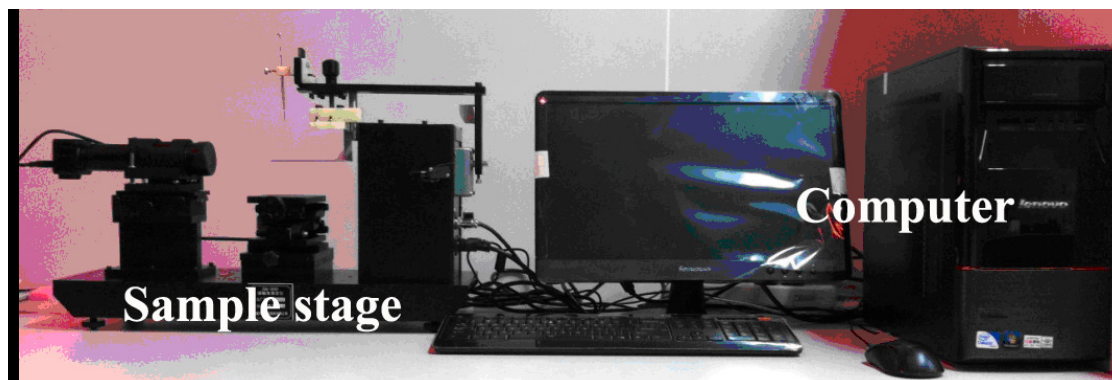
Figure 4.27 System for contact angle (CA) measurement
