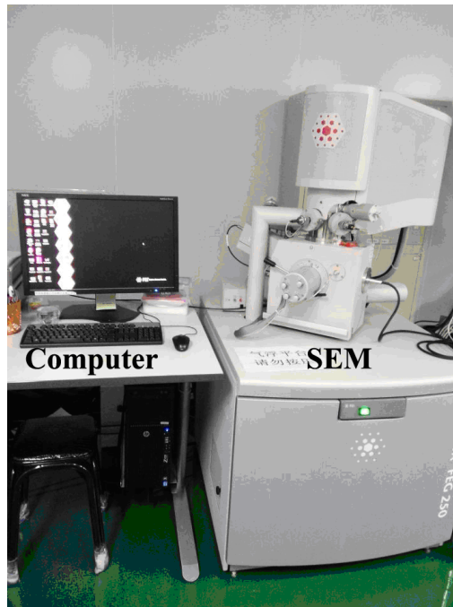
Figure 4.5 Scanning Electron Microscopy (SEM) of the FEI Quanta™ 250 in our lab.
