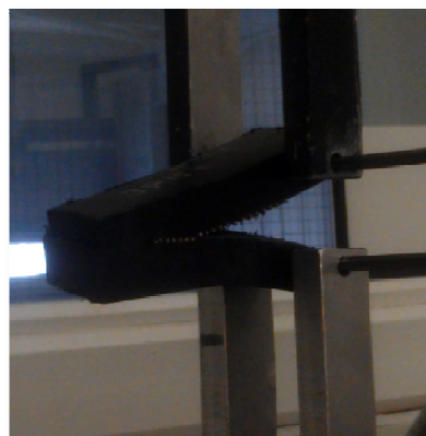
Figure 12: (Left) Instron tensile testing device (Right) Weld being pulled apart during destructive testing
