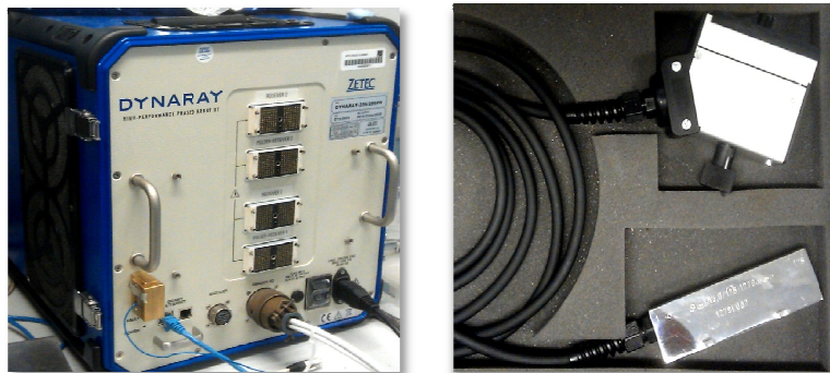
Figure 3: (Left) Zetec Dynaray phased array controller and (Right) Vermon 5MHz, 128 element probe
