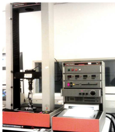
Figure 12: (Left) Instron tensile testing device (Right) Weld being pulled apart during destructive testing
