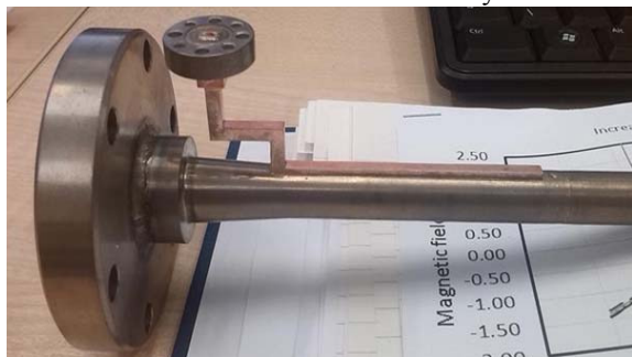
Fig. 4 A photo of the upgraded input coupler.
