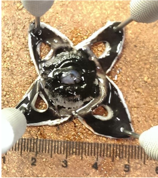
Figure 4.47 Dissected eye sample shortly after samples for permeation have been cut out of it using circular trephine.
