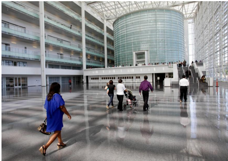
Figure 1.10 Direct sunlight from atrium glazed roof of the Sandra Day O'Connor Federal Courthouse (Santos, 2012)
