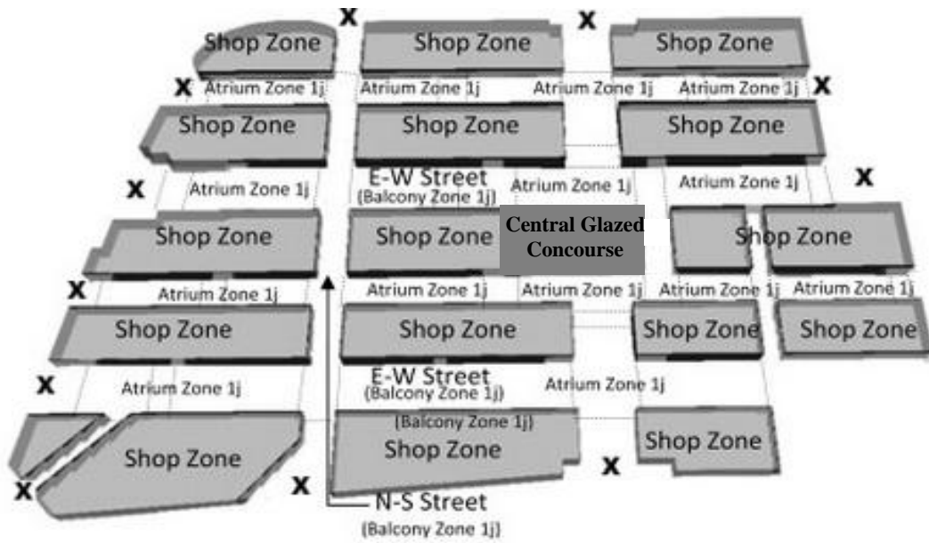
a) A ground floor plan of the building showing the central glazed spaces, indoor streets and model zoning i = \text{location } 1, 2, \dots, 22 and j = \text{floor } 1, 2, \dots, 7
