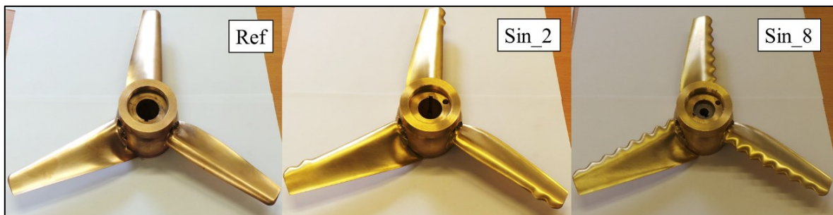
Figure 6 Tested turbine models (Left: Reference turbine with no tubercles; Middle: Turbine with partial LE tubercles; Right: Turbine with full LE Tubercles)
