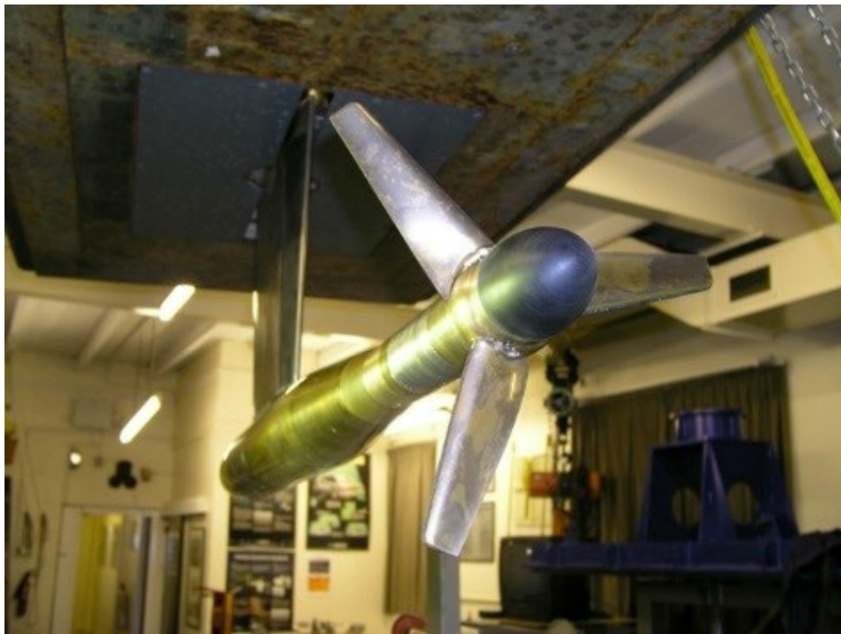
Figure 2 Scaled tidal turbine model mounted on the dynamometer of Emerson Cavitation Tunnel [19]
