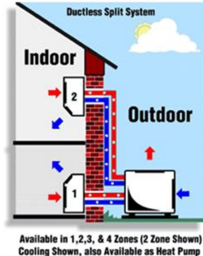
Figure 4.3: Split air conditioner system (ECR International 2015).
