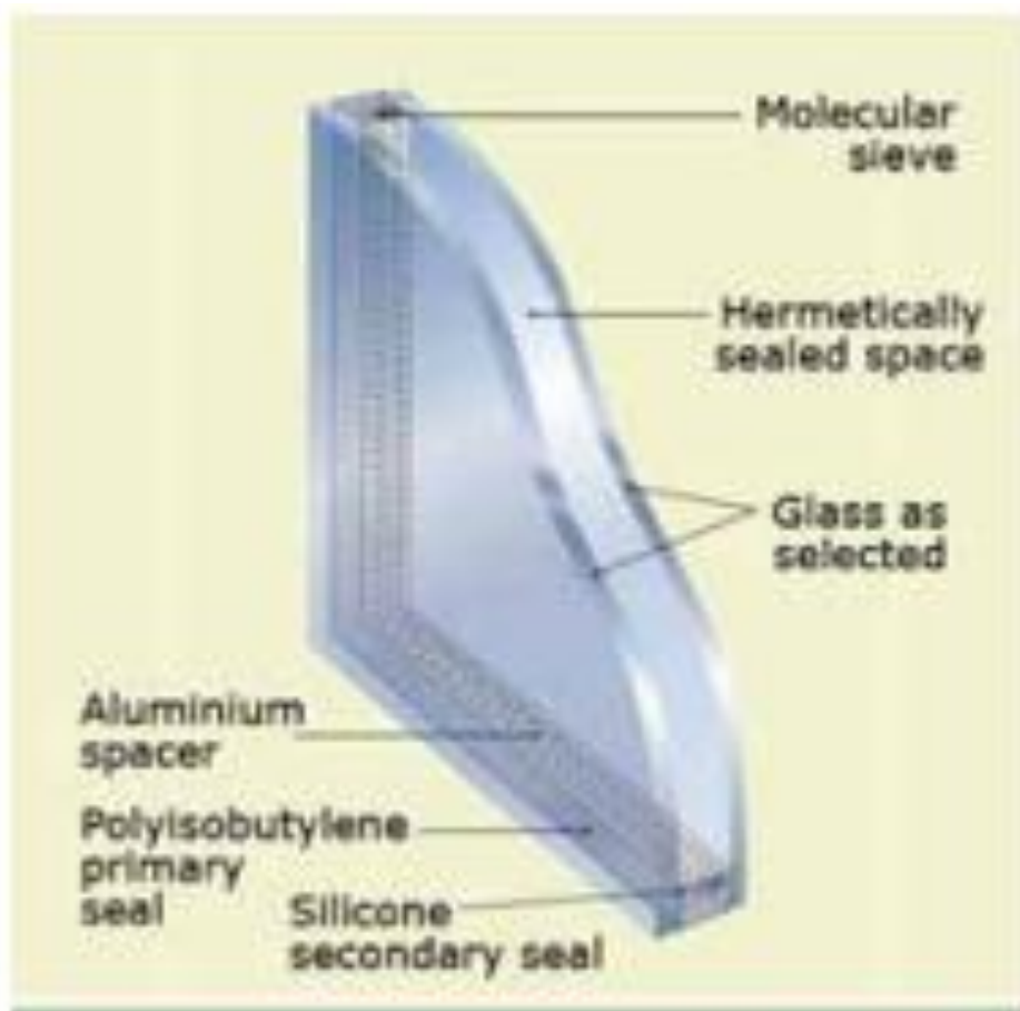
Figure 2.16: Double glazing (NEP Energy Services, 2013).
