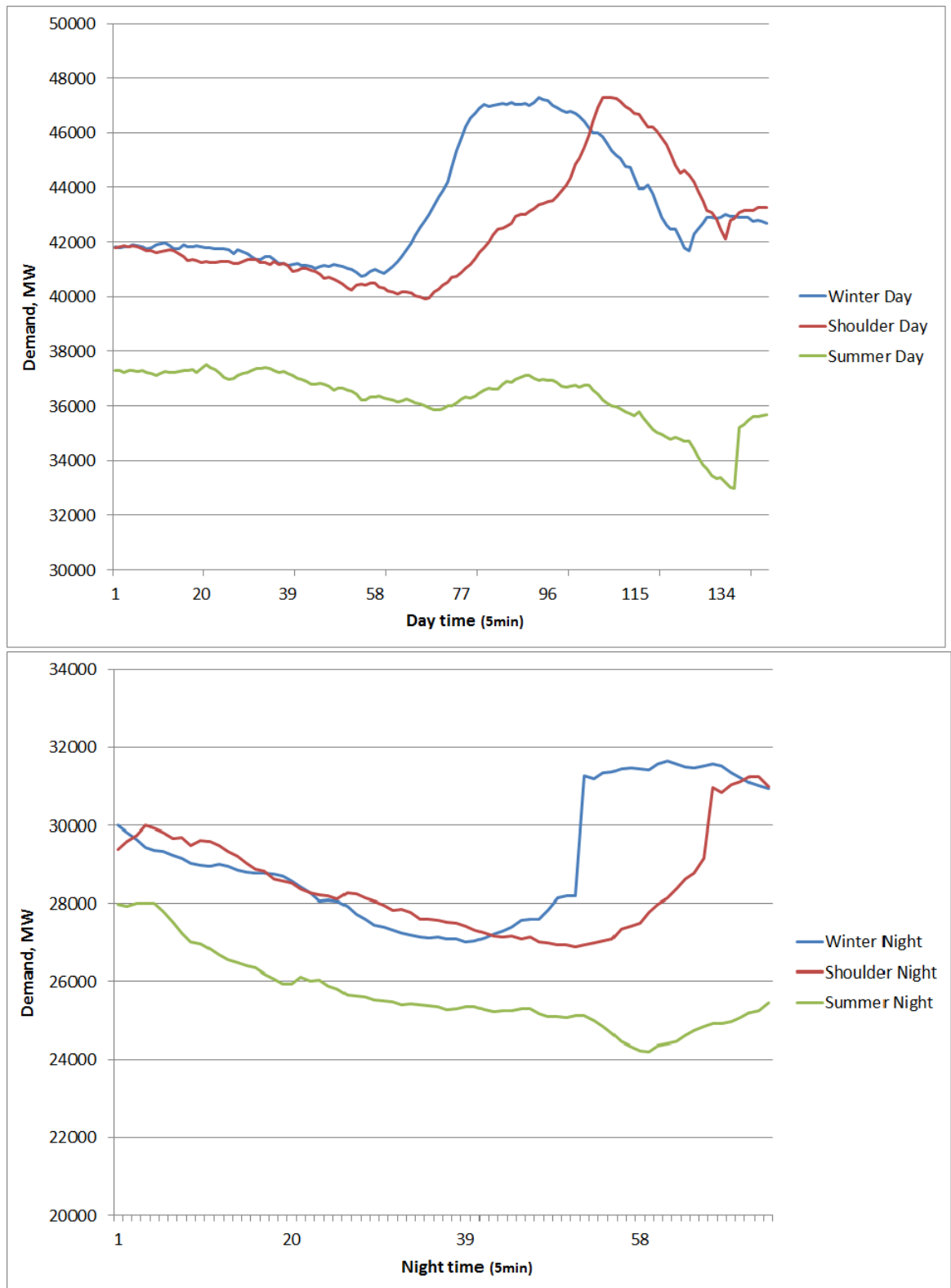
Figure 5.2: Average UK 5-min net demand for weekdays during day hours (up) and night hours (down) for each season.
