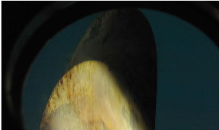
Fig. 6 – Full-scale trial cavitation observation – 600 engine rpm.
