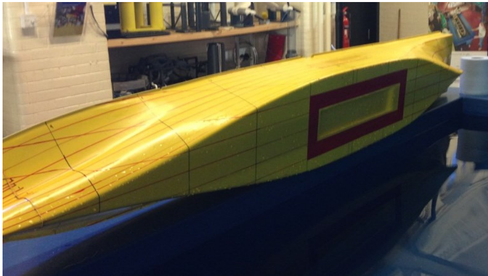
Figure 2 Air cavity accommodated on the bottom of the hull – cavity parameters can be found in Table 2.
