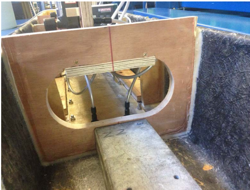
Figure 4 Air inlets into the top of the cavity
