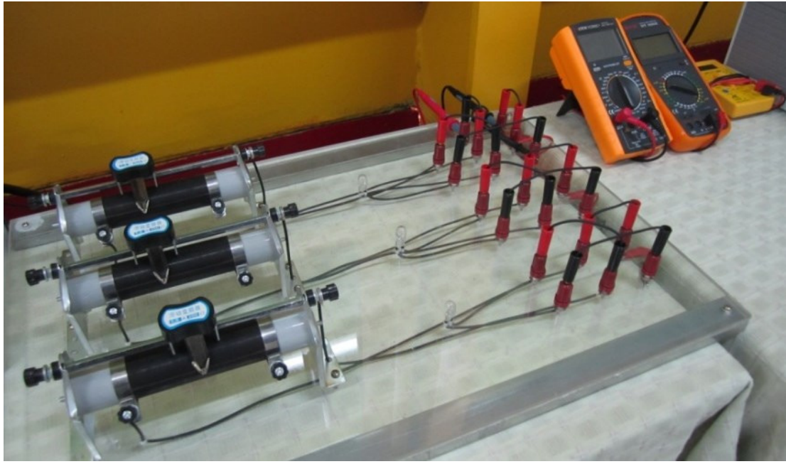
Fig.15 Rheostats for loading control
