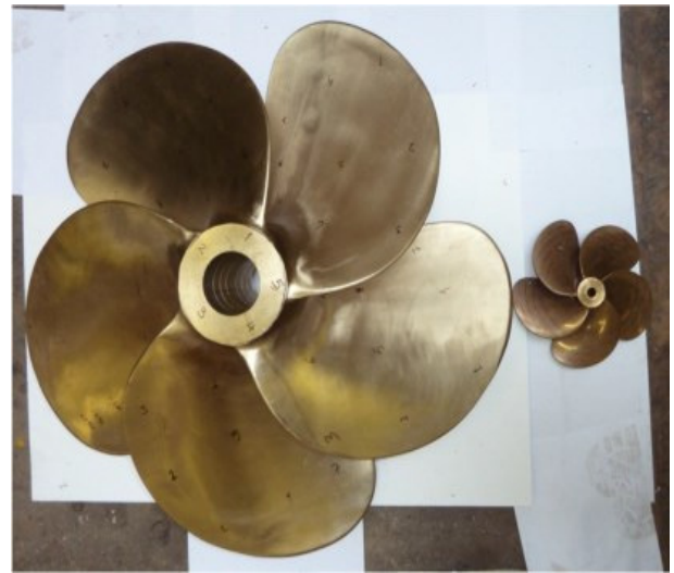
Figure 4 Views of full-scale (port) and model-scale (starboard) propellers of The Princess Royal
