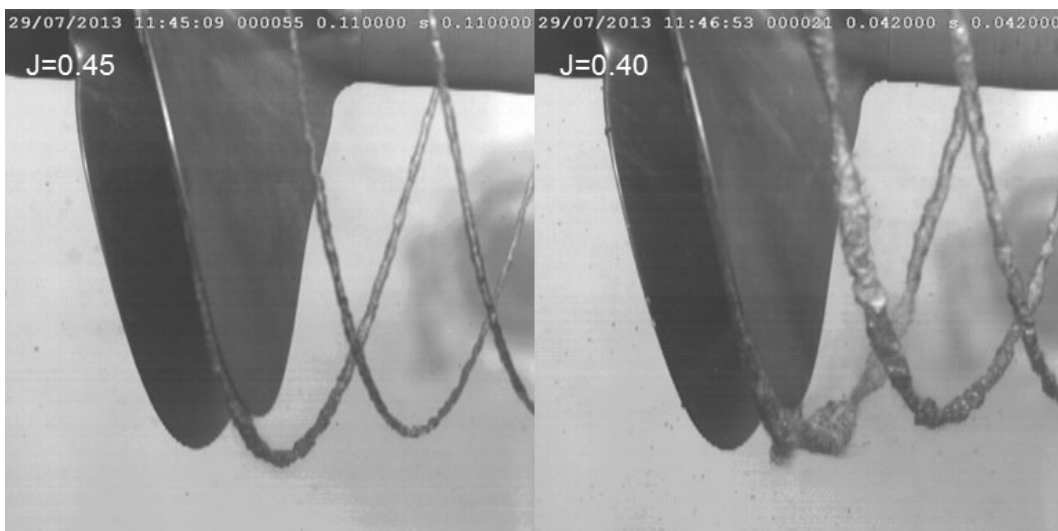
Figure 19 Cavitation patterns at 6^\circ inclination angle under medium vacuum condition
