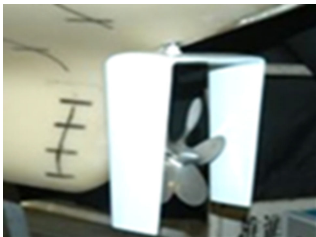
Fig. 3 Model gate rudder fitted to ship model
