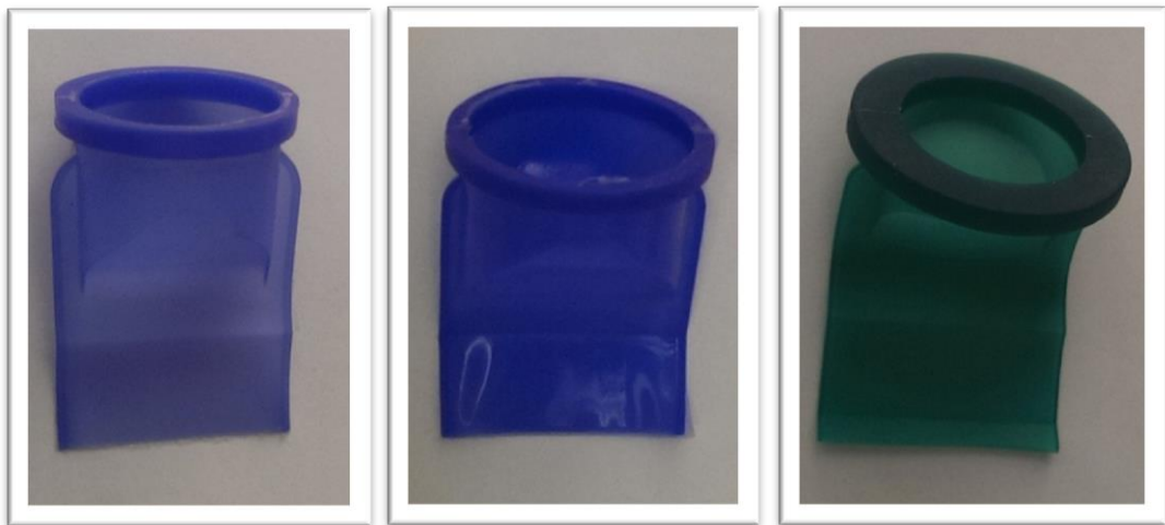
Figure 4. 15, The reference waterless trap seals, Sample 1 (left), Sample 2 (middle), and Sample 3 (right).
