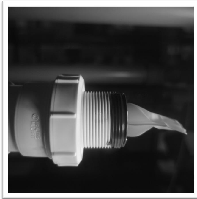
Figure 4. 18, Sample 1 connected to the 50mm pipe using a pipe fitting and adaptor
