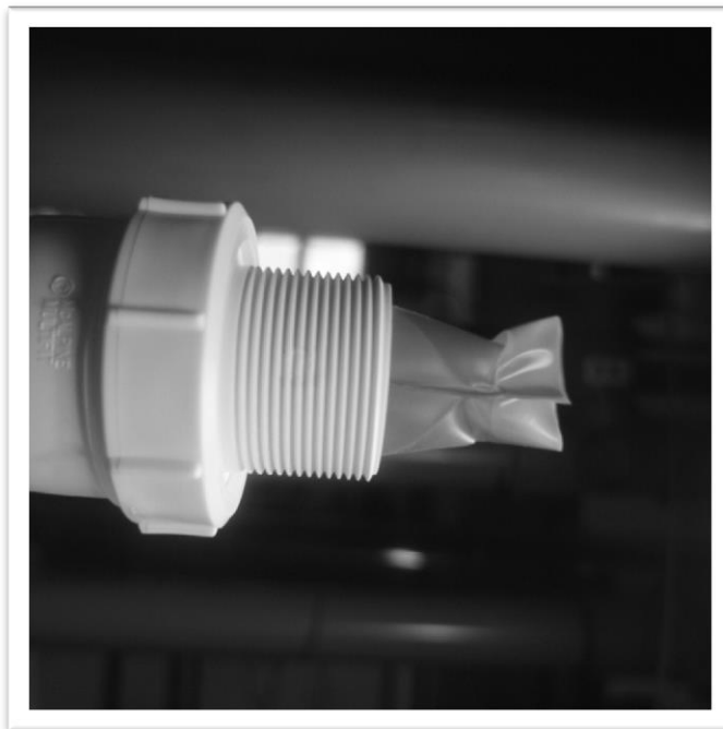
Figure 4. 19, Sample 2 connected to the 50mm pipe using a pipe fitting
