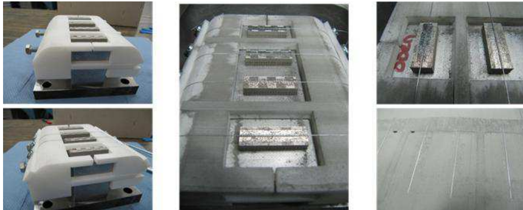
Figure 7-4 In-lets for adaption of the fibre embedding process in an commercial SLM machine. (from Inspire AG)
