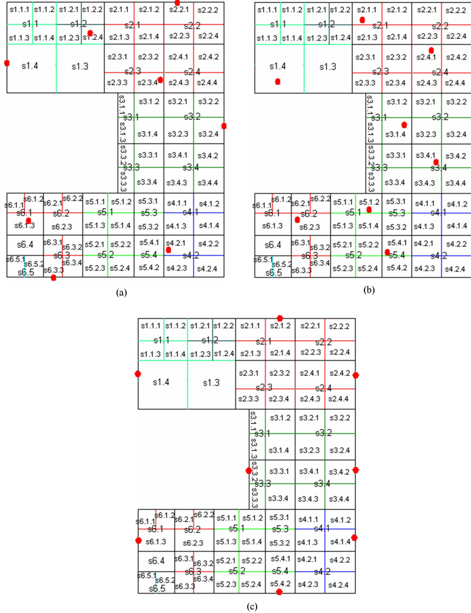
Figure 4.7: Selection of 8 fiducial points (a) at both boundary of the embryo part and inside the embryo part (b) inside the embryo part (c) at the boundary of the embryo part.
