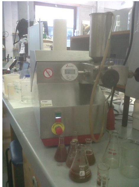
Figure 4-5. High pressure homogeniser used for the experiments.
