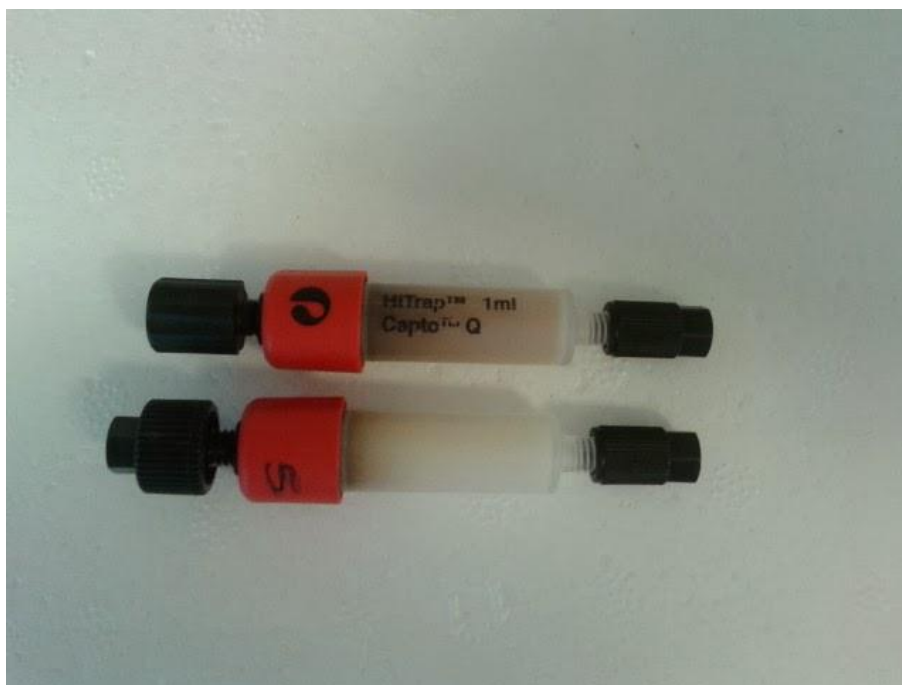
Figure 6-12. HiTrap Capto Q (up) and HiTrap Capto S (down) columns after 4 consecutive experiments.
