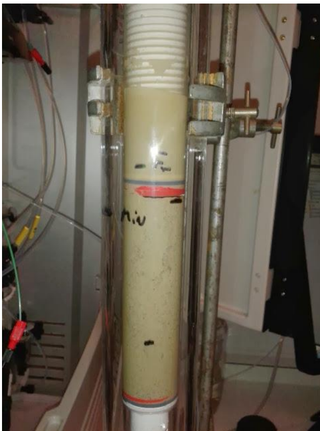
Figure 8-4. Photography of the column used during the experiments packed with zeolite as the adsorbent material.
