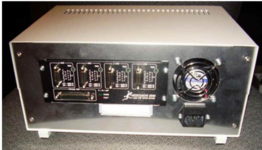
Figure 4.8 – Replacement CNC machine controller
