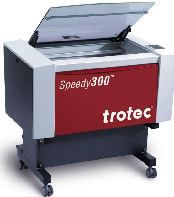
Figure 3.7 – Trotec Speedy 300 CO2 Laser engraving machine
