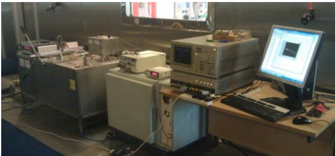
Figure 6.17. Picture of new high pressure diesel test rig. From left, diesel compression rig, oven containing test cell, impedance analyzer and PC for recording data.
