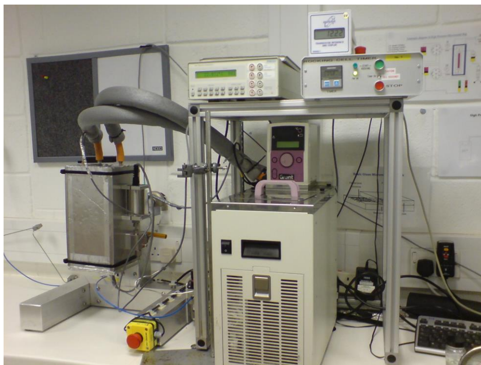
Figure 3.21. Schematic illustration of hydrate equilibrium rig used in this study, mixing ball shown was not used in this study.
