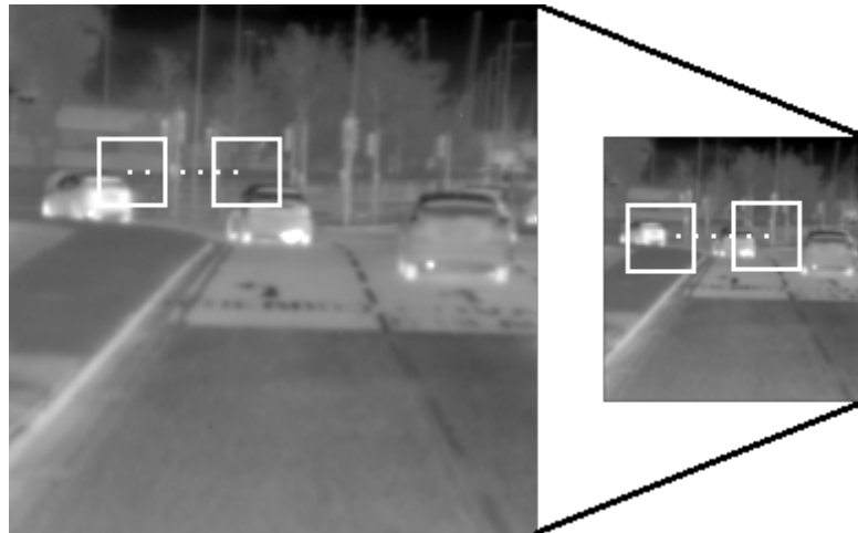
Figure 5.1: The input imagery is resized to a number of scales and for each scale a fixed size sliding window is passed spatially over the whole image. A descriptor is calculated and classified for each sliding window location.
