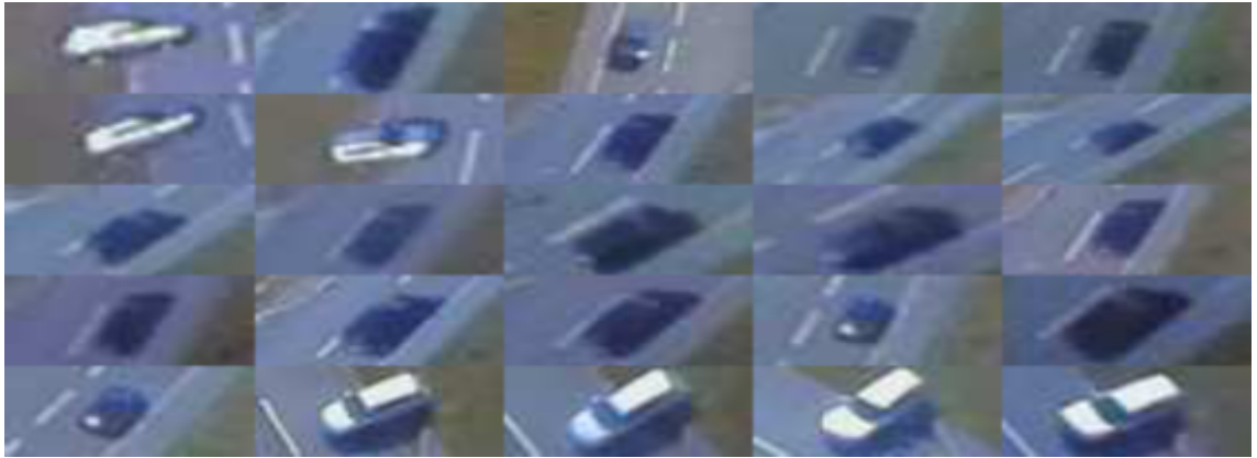
Figure 4.3: Classifiers built from Haar-like cascades are not invariant to rotation. To overcome this Breckon et al. [60] split their vehicle training set into four based on the positional orientation to the horizontal. Shown is a subset of positive samples used to train the 135^\circ classifier. (Reproduced from [60, Figure 2] © 2009 IEEE.)
