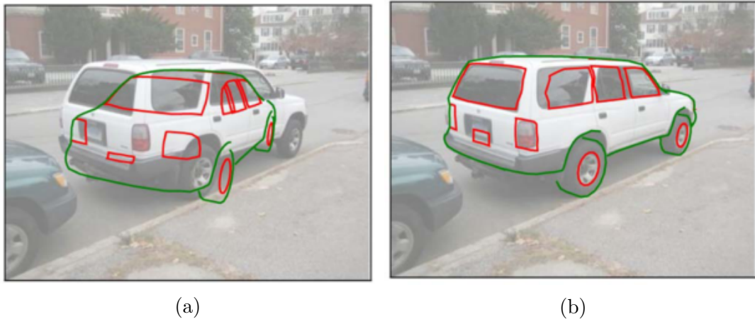
Figure 4.9: An example of hypothesised model edges projected onto images (a) before, and (b) after the fitting process. Note that both the pose and shape of the model have been optimised to match the imagery. (Adapted from [47, Figure 9] © 2010 IEEE.)
