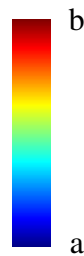
Figure 5.19: Jet colour map. The notation \text{Jet}(a,b) is used to represent values scaled between a and b
