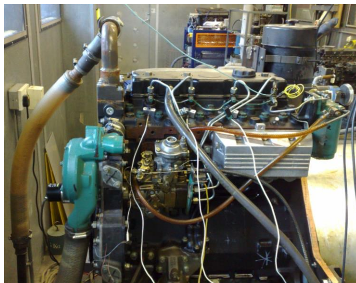
Figure 4.3: Perkins T1004 diesel engine (Engine C).
