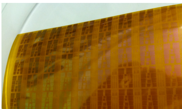
Figure 3.14: Test structures showing an increasing silver colour with increasing UV exposure time from left to right of 1 hour to 4 hours.
