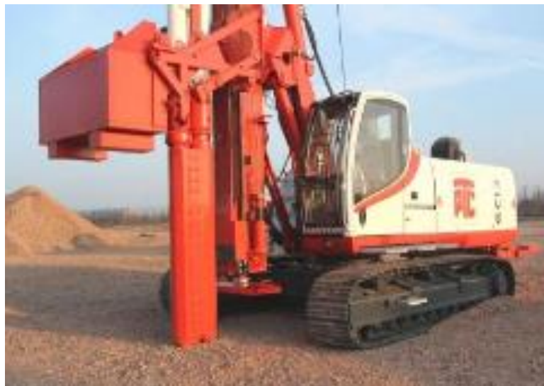
Figure 2.1 Vibro rig for installation of bottom feed stone columns (Fayat, 2013)
