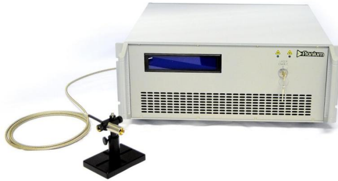
Figure 3.2 Picture of the Fianium, 6-400-PP, 6W supercontinuum laser with fibre and collimator output, which allows good optical coupling to the AOTF-HP (not shown here).
