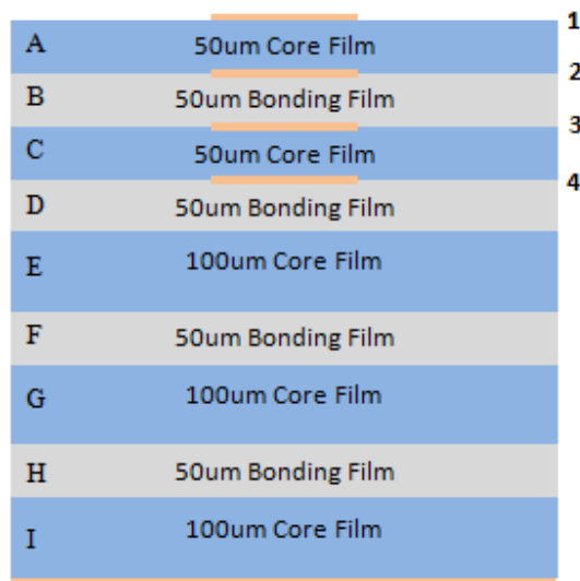
Fig. 2.13 Multilayer LCP structure for the implementation of filters in this chapter
