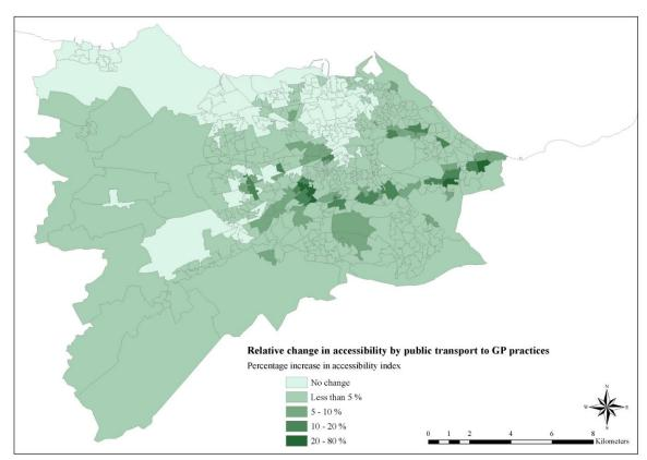
Figure D.40: Relative change in accessibility by public transport to GP practices between the baseline year 2011 scenario and Scenario I, using the potential accessibility measure
