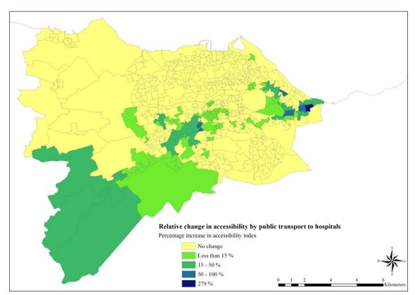
Figure D.44: Relative change in accessibility by public transport to all hospitals between the baseline year 2011 scenario and Scenario H, using the potential accessibility measure
