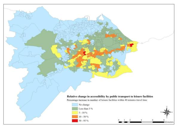
Figure C.52: Relative change in accessibility by public transport to leisure facilities between the baseline year 2011 scenario and Scenario H, using the contour measure
