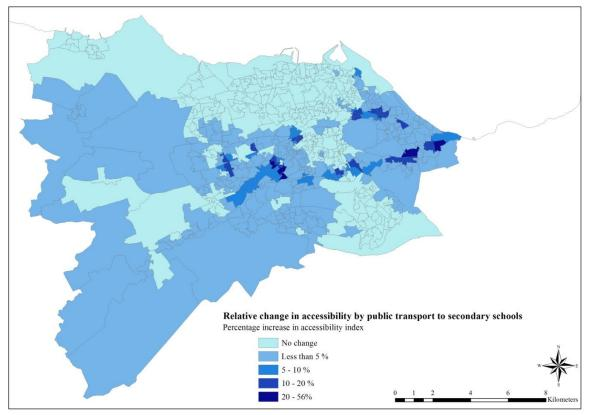
Figure D.23: Relative change in accessibility by public transport to secondary schools between the baseline year 2011 scenario and Scenario H, using the potential accessibility measure
