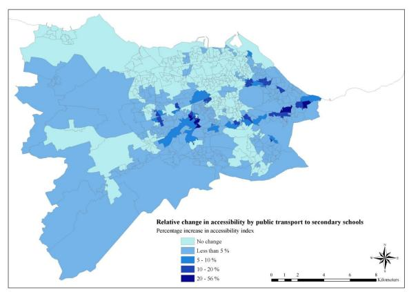
Figure D.24: Relative change in accessibility by public transport to secondary schools between the baseline year 2011 scenario and Scenario I, using the potential accessibility measure
