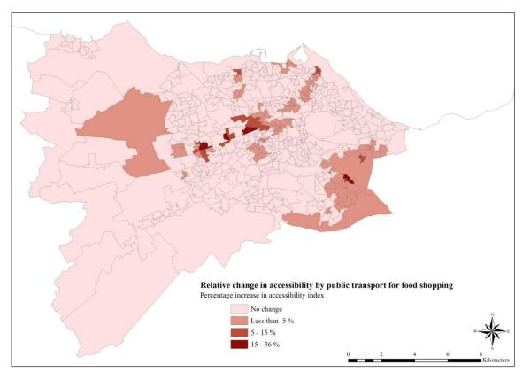
Figure D.6: Relative change in accessibility by public transport to food stores between the baseline year 2011 scenario and Scenario G, using the potential accessibility measure
