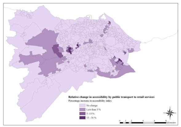
Figure D.13: Relative change in accessibility by public transport to retail services between the baseline year 2011 scenario and Scenario F, using the potential accessibility measure
