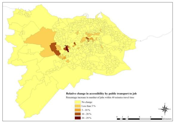
Figure C.3: Relative change in accessibility by public transport to jobs between the baseline year 2011 scenario and Scenario E, using the contour measure
