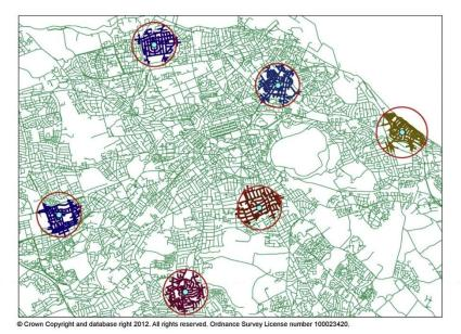
Fig. 4. Map showing how a multiplier of 1.2 is estimated based on a few example points around the city of Edinburgh with 800 m actual distance and 670 m radius circles. *Source:* City of Edinburgh Council, Services for Communities.
