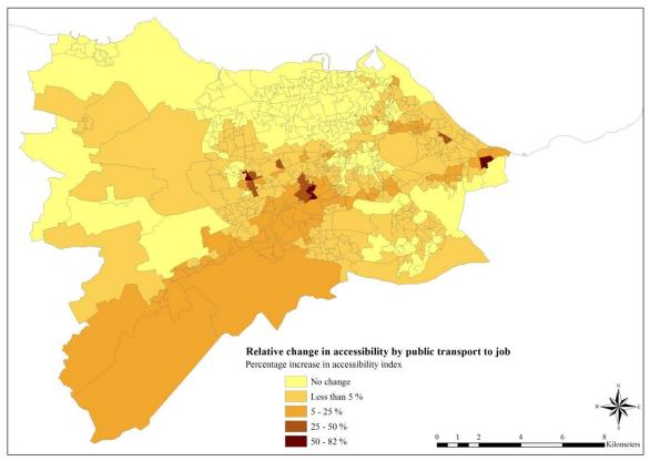
Figure 7.39: Relative change in accessibility by public transport to jobs between the baseline year 2011 scenario and Scenario H, using the potential accessibility measure
