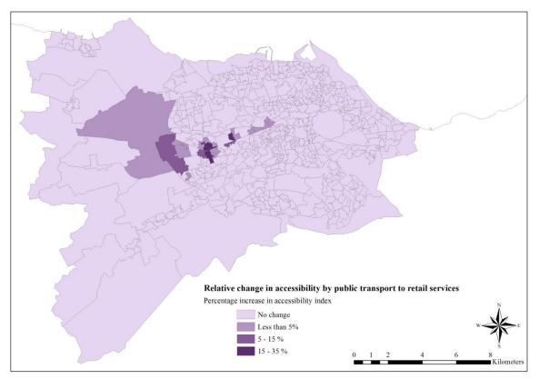
Figure D.9: Relative change in accessibility by public transport to retail services between the baseline year 2011 scenario and 2014 scenario (Scenario B), using the potential accessibility measure
