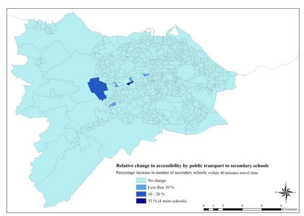
Figure C.24: Relative change in accessibility by public transport to secondary schools between the baseline year 2011 scenario and Scenario E, using the contour measure
