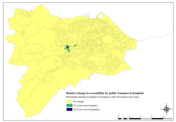
Figure C.43: Relative change in accessibility by public transport to all hospitals between the baseline year 2011 scenario and Scenarios C, D, E, F and G, using the contour measure
