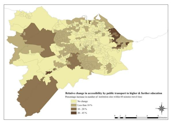
Figure C.34: Relative change in accessibility by public transport to higher & further education facilities between the baseline year 2011 scenario and Scenario H, using the contour measure
