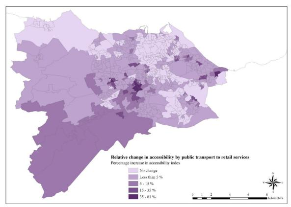
Figure D.16: Relative change in accessibility by public transport to retail services between the baseline year 2011 scenario and Scenario I, using the potential accessibility measure
