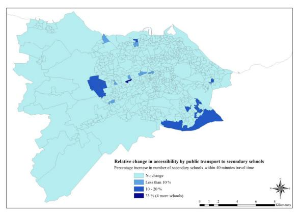
Figure C.26: Relative change in accessibility by public transport to secondary schools between the baseline year 2011 scenario and Scenario G, using the contour measure
