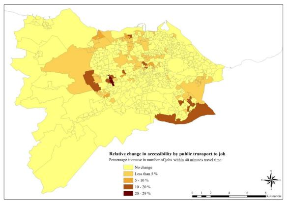
Figure C.5: Relative change in accessibility by public transport to jobs between the baseline year 2011 scenario and Scenario G, using the contour measure
