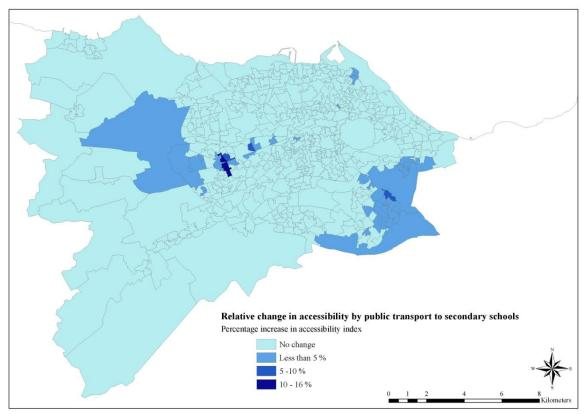
Figure D.21: Relative change in accessibility by public transport to secondary schools between the baseline year 2011 scenario and Scenario F, using the potential accessibility measure
