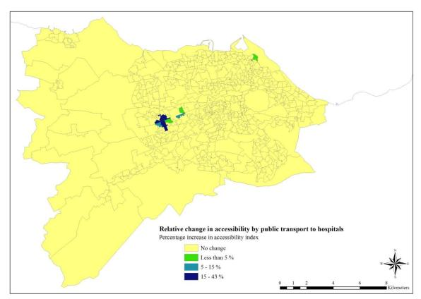
Figure D.42: Relative change in accessibility by public transport to all hospitals between the baseline year 2011 scenario and Scenarios C, D and E, using the potential accessibility measure
