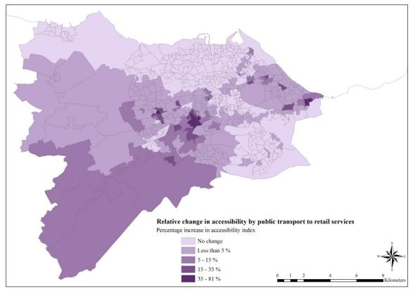
Figure D.15: Relative change in accessibility by public transport to retail services between the baseline year 2011 scenario and Scenario H, using the potential accessibility measure
