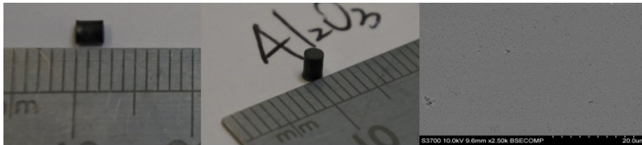
Figure 5 . A formed sample (solid cylinder) with a size of \Phi 2.0mm \times 2.0mm and its SEM micrograph
