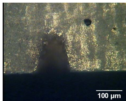
Figure 3.3.2. Laser machined lines measured with optical microscope. The image represents a side view of the specimen.
