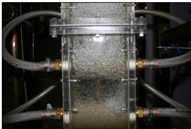
Figure 3.10: Bubble generator in operation
