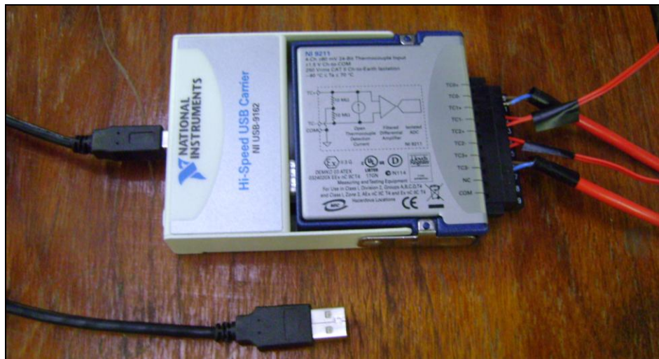
Figure 3.31: Thermocouple input Module NI USB-9211A
