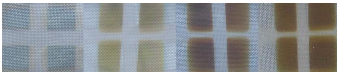
Figure 6.4. Deposition visually changed in thickness with increased silane rate (0.10, 0.51, 1.02 and 2.04sccm), when image to the left (0.10sccm) has very thin deposition compared with the films to follow, which have higher silane rate (0.51, 1.02 and 2.04sccm moving to the right). All samples had H_2/Ar ratio of 17/3sccm.
