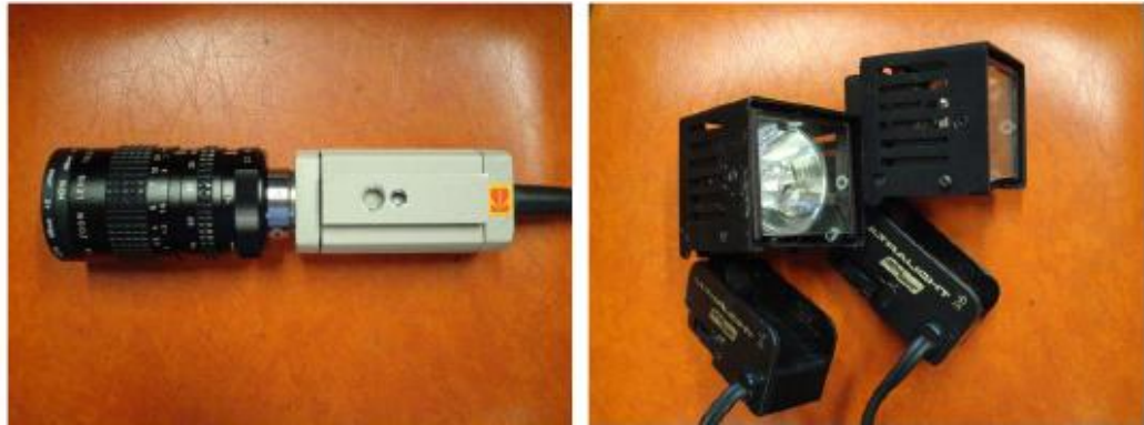
Figure 3.5: High speed video camera and the lighting systems
