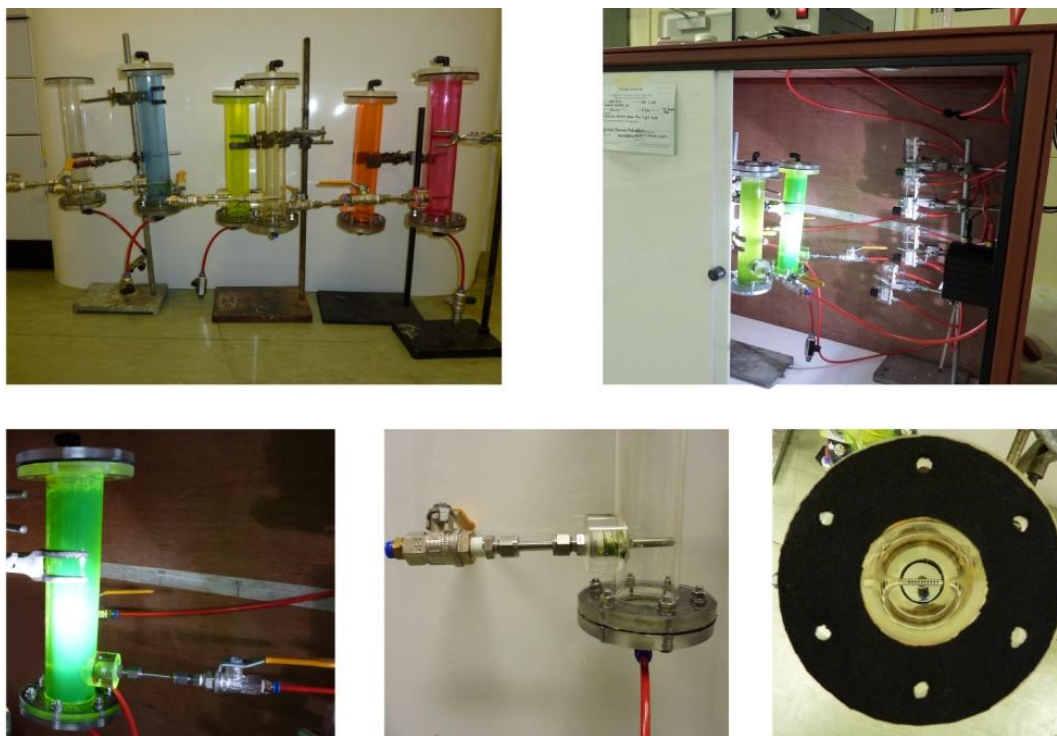
Figure 3.7, Left to right clockwise: Luminescent PBR in six different ranges, PBR in operation inside the light box, top view of the PBR, side views of the PBR.
