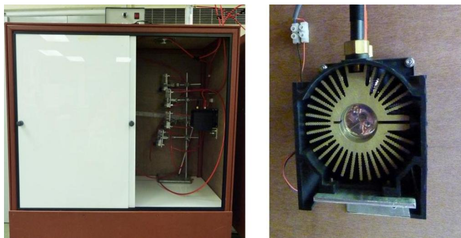
Figure 3.3, Light box (left side) equipped with xenon lamp (right side) used in this study for illumination of cultures either in static or aerated modes.
